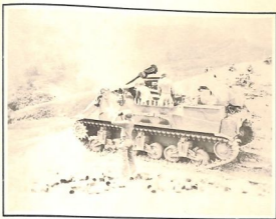
A self-propelled howitzer (M-7) fires in support of mop-up troops beyond the next ridge.
