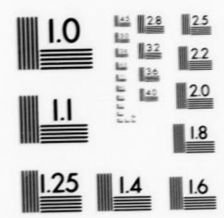
MICROCOPY RESOLUTION TEST CHART NATIONAL BUREAU OF STANDARDS STANDARD REFERENCE MATERIAL 1010s (ANSI and ISO TEST CHART No. 2)
